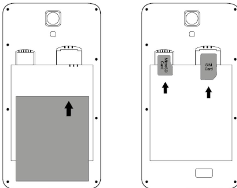
The above diagram shows the locations for Standard SIM card, battery and the Micro SD card
